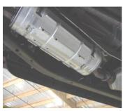
TO REMOVE STOCK EXHAUST UNBOLT IT FROM THE SLIP-FIT JOINT LOCATED IN THE REAR ABOVE THE AXLE AND SLIDE THE TAILPIPE OUT. NEXT UNBOLT THE 2-BOLT FLANGE LOCATED JUST BEHIND THE CATALYTIC CONVERTER. DO NOT THROW **AWAY STOCK NUTS AND BOLTS YOU WILL NEED TO RE-USE THEM.** NOW CUT OFF YOUR STOCK TAILPIPE JUST BEHIND THE MUFFLER AND REMOVE. LEAVE ALL RUBBER GEOMMETS ON THE HANGER. USE WD-40 TO AID IN THE REMOVAL OF EXHAUST AND HANGERS.
