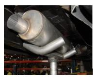
INSTALL MUFFLER #C ONTO TAILPIPE 1-1/2" TO 2" WITH INLET TOWARDS THE MOTOR. USE CLAMP #G TO SECURE THE TAILPIPE AND THE MUFFLER, DO NOT TIGHTEN. MUFFLER INLET SHOULD BE AT 9 O'CLOCK POSITION.
