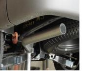
INSTALL EXIT PIPE #E AND INSERT WELDED HANGER INTO RUBBER GROMMET.
