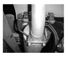
INSTALL REAR MUFFLER HANGER # D ON TO THE OUTLET OF THE MUFFLER AND INSERT WELDED RODS INTO RUBBER GROMMET. THE VERTICAL ROD'S ON THE HANGER WILL BE FACING TOWARDS THE PASSENGER SIDE. DO NOT TIGHTEN.
