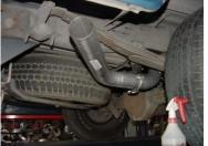
INSTALL THE TURNOUT PIPE #D ONTO THE TAILPIPE #C. SECURE TOGETHER WITH CLAMP #I. DO NOT TIGHTEN. ROLL THE TURNOUT PIPE UNTIL IT IS AT THE CORRECT LEVEL FOR YOUR TRUCK.
