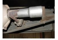
LONG BEDS: INSTALL HEADPIPE #A ONTO YOUR EXISTING HEADPIPE AND SECURE WITH CLAMP #F. DO NOT TIGTHEN.
