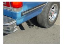
INSTALL THE STAINLESS TIP. TO CLEAN TIP USE ANY STAINLESS CLEANER AND A SCOTCH BRITE PAD. NOW GO BACK AND TGHTEN ALL CLAMPS STARTING FROM THE FRONT AND WORKING BACK.
