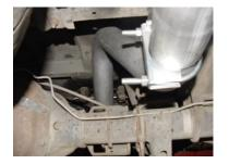
INSTALL THE OVERAXLE TAILPIPE #C INTO THE MUFFLER 1-1/2" TO 2". SECURE TO THE MUFFLER USING CLAMP #I. SLIDE HANGER #H ONTO THE END OF THE TAILPIPE AND INSERT HANGER INTO RUBBER GROMMET. DO NOT TIGHTEN.
