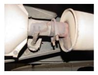
LAY OUT THE EXHAUST ON THE FLOOR SO IT LOOKS LIKE THE DRAWING AND COMPARE PARTS TO THE MANUAL. TO REMOVE STOCK EXHAUST UN-BOLT THE CLAMP LOCATED JUST BEHIND THE CATALYTIC CONVERTER. USE JACK STANDS TO SUPPORT THE CONVERTER. LEAVE ALL RUBBER GROMMETS IN PLACE. FOR EASIER REMOVAL USE WD-40 ON HANGERS.
