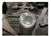
INSTALL MUFFLER #B ONTO HEADPIPE #A 1-1/2" TO 2". USE A JACKSTAND TO SUPPORT MUFFLER. SECURE MUFFLER TO HEADPIPE WITH CLAMP #I. DO NOT TIGHTEN. INSTALL HANGER #G ONTO OUTLET OF MUFFLER AND INSERT HANGERS INTO RUBBER GROMMETS. MUFFLER INLET IS LOOKING INTO THE LOUVERS.
