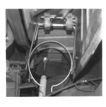
**3.** INSTALL BAND CLAMP #H AND INSERT RODS INTO RUBBER GROMMETS LOCATED JUST ABOVE THE AXLE AND ATTACH WITH BOLT KIT # I.
