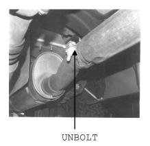
1. LAY OUT THE EXHAUST SYSTEM SO IT MATCHES THE DRAWING. MAKE SURE ALL PART NUMBERS ARE CORRECT, UNBOLT THE WELDED MUFFLER ASSEMBLY IN FRONT OF THE MUFFLER. DO NOT REMOVE THE **EXTENSION PIPE BEHIND** THE CONVERTER. FOR AN EASIER REMOVAL OF THE FACTORY EXHAUST. CUT THE TAILPIPE JUST BEHIND THE FACTORY MUFFLER. LEAVE ALL RUBBER GROMMETS IN PLACE. USE WD-40 FOR EASIER REMOVAL OF FACTORY HANGER.
