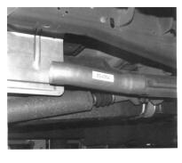
2. INSTALL HEADPIPE #A ONTO THE FACTORY EXTENSION PIPE. USE CLAMP #E TO ATTACH IT TO THE FACTORY EXTENSION PIPE. DO NOT TIGHTEN
