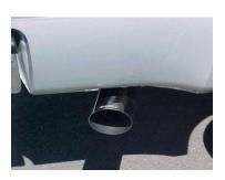
Install the over axle tailpipe # C into the muffler 1-1/2" to 2". Secure to the muffler using clamp # G Do not tighten.
