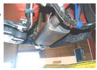
4. Now do the same procedure for the driver side tailpipes. Use clamp # C to secure the tailpipe to the muffler and stock clamp to secure it to the stock h-pipe.
