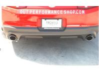
5.When you have everything in Place, firmly tighten all bolts And clamps down securely Use stainless steel cleaner and Scotch Brite pad weekly to prevent tip from discoloration. Inspect all fasteners after 25-50 miles of operation and re-Tighten as necessary
