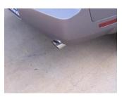
**4.** Install stainless steel tips. Clamp down. When you have everything in place, firmly tighten all bolts and clamps down securely. Use stainless steel cleaner and a Scotch Brite pad weekly to prevent tip from discoloration.
