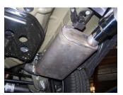
**3.** Install muffler assembly onto factory pipe, use clamp #B to secure. DO NOT TIGHTEN. Next tighten grommets to frame and adjust muffler assembly.
