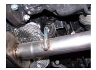
Install passenger side tailpipe/muffler assembly #C. Insert all welded hangers into rubber grommets.
