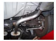
6. Install passenger side tailpipe/muffler assembly #C. Insert all welded hangers into rubber grommets. Secure tailpipe with clamp #D. Do not tighten. Now go back and make sure the first two mufflers in the middle are level.
