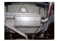
5. Now slide muffler #C onto inlet pipe 1.5-2". Secure with clamp #F, do not tighten.
