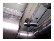
6. Next, slide exit pipe #D into muffler 1.5-2". Insert welded hanger into rubber grommet. Secure with clamp #F, do not tighten.
