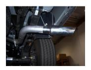
**6.** Install exit pipe #D onto overaxle tail pipe. Use clamp #F to secure. DO NOT TIGHTEN.
