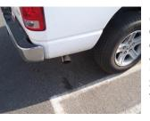
**6.** Install stainless steel tip #D. Clamp down. When you have everything in place, firmly tighten all bolts and clamps down securely. Use stainless steel cleaner and a Scotch Brite pad weekly to prevent tip from discoloration.
