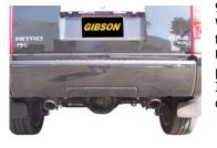
GIBSON EXHAUST systems are designed on a factory stock vehicle. Any aftermarket products installed could increase the sound levels of the exhaust. **Make sure there is a 1**" clearance from ALL rubber brake lines, shock boots, lines, tires, etc. to prevent heat related damage or fire.
