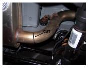
2. First remove the clamp located in front of the muffler. Disengage the welded hangers from the rubber grommets. Use WD-40 to aid in this process. Do not damage or remove the rubber grommets as you will reuse them to mount the new system. Now cut off the tailpipe and remove exhaust. Use a jack stand to support the converter.
