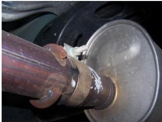
2. To remove your stock exhaust, remove the clamp located in front of the muffler. For easier removal, unbolt rear tailpipe hanger and grommet with a 13mm wrench. Then remove other hanger from rubber grommet, and cut off tailpipe just behind muffler. Now remove the rest of the system at the clamp.
