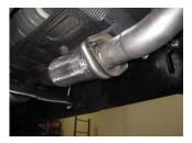
3. Install headpipe #A onto your existing stock 2-bolt flange. Use factory nuts to secure. Leave loose until the whole system is installed. Insert welded hanger into rubber grommet.
