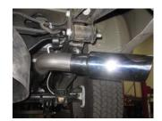
7. Install stainless steel tip. Clamp down. When you have everything in place, firmly tighten all bolts and clamps down securely. Inspect all fasteners after 25-50 miles of operation and re-tighten as necessary.
