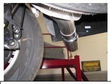
from spare tire install the exhaust tip onto the tailpipe. The system was designed to have the tip 1" below the quarter panel of the vehicle. With the tip in your desired position begin to tighten down all clamp connections from the
