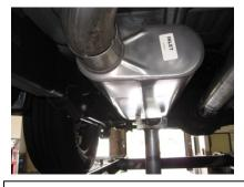
3. Install muffler #B onto headpipe 1.5" to 2" muffler should be level use clamp #E to secure together do not tighten.
