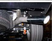
**6.** Install exit pipe #D into the tailpipe 1½-2" and secure with clamp #F. DO NOT TIGHTEN. Rotate pipe to best suit your vehicle.
