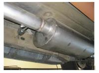
**4.** Install muffler #B onto head pipe 1½"-2" with the louvers facing towards the converter. Use a jack stand to support the muffler. Use clamp #F to secure the muffler to the headpipe. DO NOT TIGHTEN. Muffler inlet is looking into louvers.
