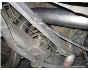
**5.** Install tailpipe #C into muffler 1½-2" and secure with clamp #F. DO NOT TIGHTEN. Insert welded hanger into rubber grommet.
