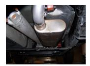
**4.** Install muffler #B onto head pipe #A. 1½"-2" with the louvers facing towards the converter. Use a jack stand to support the muffler. Use clamp #E to secure the muffler to the headpipe. DO NOT TIGHTEN. Muffler inlet is looking into the louvers. Outlet will be on the drivers side.
