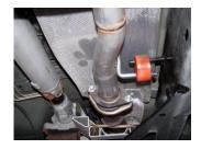
**3.** Install head pipe #A onto your existing stock front pipe and attach with bolt kit #F. Insert welded hanger into rubber grommet.
