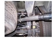
**5.** Install tailpipe #C into the muffler 1½-2". Insert welded hangers into rubber grommets use clamp #E to secure to muffler. Do not tighten.
