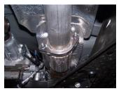
**2.** To remove the stock exhaust remove it from the flange located in front of your stock muffler. Disengage the welded hangers using WD-40 from the OEM rubber grommets. Do not damage or remove the rubber grommets as you will re-use them to mount your new system. Now, cut off tailpipe and remove exhaust.
