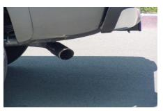
INSTALL THE STAINLESS TIP. TO CLEAN TIP USE ANY STAINLESS OR ALUMINUM CLEANER AND A SCOTCH BRITE PAD.
