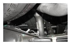
AFTER YOU HAVE CHECKED FOR PROPER CLEARANCES YOU CAN TIGHTEN ALL CLAMPS STARTING FROM THE FRONT AND WORKING YOUR WAY BACK.
