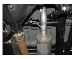
INSTALL TAILPIPE #D INTO MUFFLER 1-1/2" TO 2". INSERT WELDED HANGER INTO RUBBER GROMMET. USE CLAMP #H TO SECURE TAILPIPE #D TO MUFFLER. DO NOT TIGHTEN.
