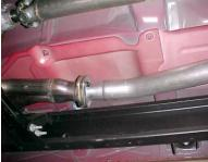
BOLT HEADPIPE #A TO THE STOCK FLANGE RE-USING THE FACTORY NUTS & BOLTS. INSERT WELDED HANGER INTO RUBBER GROMMET.
