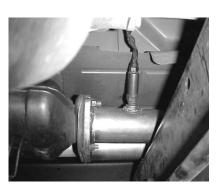
RE-INSTALL O2 SENSOR. USE A SMALL AMOUNT ANTI-SIEZE ON THE THREADS. NOW FIRMLY TIGHTEN ALL CLAMPS, HANGERS, FLANGE, AND BOLTS.
