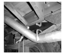
INSTALL THE OVERAXLE TAILPIPE #C INTO MUFFLER AT LEAST 1 1/2" TO 2" USING CLAMP #G. DO NOT TIGHTEN. INSERT WELDED HANGERS INTO RUBBER GROMMETS. THE SPARE TIRE ON SOME VEHICLES MAY NEED TO BE LOOSEN AND PULLED TO THE DRIVER SIDE AND RE-TIGHTENED. ROTATE PIPES UNTIL YOU HAVE AT LEAST A 1" CLEARANCE AWAY FROM SHOCK, BRAKE LINES, SPARE TIRE ECT.
