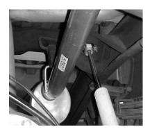
SLIDE MUFFLER WITH DUAL INLET ONTO HEADPIPE AT LEAST 1-1/2" TO 2".
