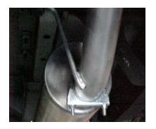
SLIDE MUFFLER WITH DUAL INLET ONTO HEADPIPE AT LEAST 1-1/2" TO 2". MUFFLER OUTLET SHOULD BE AT THE 6 O'CLOCK POSITION. USE CLAMPS #F TO ATTACH IT TO THE HEADPIPE. INSERT WELDED HANGER INTO RUBBER GROMMET. MAKE SURE INLETS AND MUFFLER IS LEVEL. AND TIGHTEN DOWN. USE JACK STAND TO SUPPORT MUFFLER.
