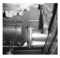
REMOVE O2 SENSOR FROM STOCK HEAD PIPE AND UN-BOLT STOCK HEAD-PIPE. YOU WILL REUSE YOUR STOCK NUTS AND BOLTS. CUT STOCK EXHAUST JUST BEHIND THE MUFFLER FOR EASIER REMOVAL. LEAVE ALL RUBBER GROMMETS IN PLACE. FOR EASIER REMOVAL OF THE HANGERS SPRAY WD-40 TO AID YOU IN REMOVING THEM.
