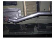
**5.** Install the overaxle tailpipe #C to the muffler  $1\frac{1}{2}$ -2". Use clamp #E to secure tailpipe to muffler. Insert welded hanger into rubber grommet.
