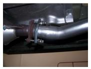
2. To remove the stock exhaust, unbolt the 2 bolt flange located in front of the new muffler. Disengage the welded hangers using WD-40 from the OEM rubber grommets. Do not damage or remove the rubber grommets as you will reuse them to mount your new system. Now, cut off tailpipe and remove exhaust.
