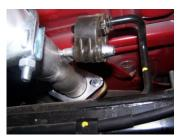
3. Install headpipe #A onto vour existing stock flange using bolt kit #F to secure flange, DO NOT TIGHTEN. Insert welded hanger into rubber grommet.
