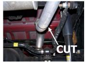
5. Install tailpipe #C into muffler approximately 11/2-2". Secure tailpipe with clamp #E. DO NOT TIGHTEN. Insert welded hanger into rubber grommet.
