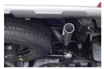
INSTALL EXITPIPE #D ONTO OVERAXLE TAILPIPE. INSERT WELDED HANGERS INTO RUBBER GROMMETS. USE CLAMP #H TO SECURE TO THE TAILPIPE. DO NOT TIGHTEN.
