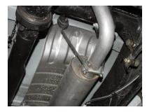
INSTALL HANGER #G INTO RUBBER GROMMET LOCATED JUST ABOVE THE OUTLET OF THE MUFFLER. USE THIS HANGER TO SECURE MUFFLER TO TAILPIPE. DO NOT TIGHTEN.
