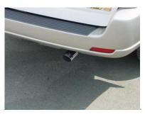
INSTALL THE STAINLESS TIP #E. TO CLEAN TIP USE ANY STAINLESS OR ALUMINUM CLEANER AND A SCOTCH BRITE PAD. NOW GO BACK AND TIGHTEN ALL NUTS, BOLTS AND CLAMPS STARTING FROM THE FRONT AND WORKING BACK.
