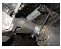
INSTALL FRONT MUFFLER HANGER #F INTO RUBBER GROMMETS LOCATED JUST ABOVE THE INLET OF THE MUFFLER. USE THIS CLAMP TO SECURE HEADPIPE. DO NOT TIGHTEN.
