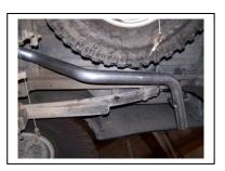
Install the over axle tailpipe # C into the muffler 1-1/2" to 2". Secure to the muffler using hanger # D. Do not tighten.
