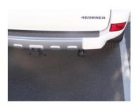
Install stainless steel tip. Clamp down. When you have everything in place, firmly tighten all bolts and clamps down securely. To clean stainless steel cleaner and Scotch Brite pad.
