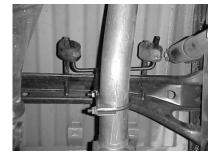
INSTALL HANGER #DINTO THE REAR MUFFLER RUBBER GROMMETS. THE VERTICAL RODS WILL BE FACING TOWARDS THE REAR OF THE TRUCK.
