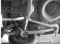
SLIP THE OVER AXLE PIPE #C INTO THE OUTLET OF THE MUFFLER NO MORE THEN 2" AND NO LESS THEN 1". USE CLAMP # E TO SECURE TAILPIPE TO MUFFLER. DO NOT TIGHTEN. INSERT WELDED HANGER INTO RUBBER GROMMET.
