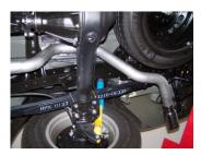
7. Install the overaxle tailpipe #E to the rear extension pipe #D. Use clamp #H to secure pipe. Do not tighten. Install hanger into rubber grommet.
