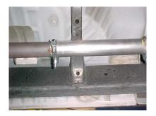
SLIDE THE HEADPIPE ONTO THE STOCK HEADPIPE ATTACHING CLAMP # E.
