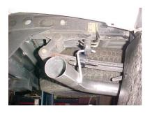
INSTALL WELDED HANGER INTO GROMMET.
