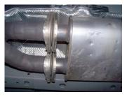
2. To remove the stock exhaust, unbolt the tailpipes at the clamps behind the over axle pipe. Then disengage hangers from the rubber grommets, and remove the rear tailpipes and mufflers. Now remove all other hangers from rubber grommets and unbolt the rest of the exhaust system at the 2 flanges in front of the stock muffler.
