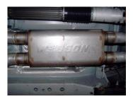
4. Install muffler #C onto headpipes 1.5-2". Use a jack stand to support muffler. Use clamp #G to attach muffler to headpipes. Do not tighten.
