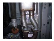
3. Install passenger side headpipe #A onto stock flanges using bolt kit #H. Do not tighten. Then install driver side headpipe #B using bolt kit #H. Do not tighten.
