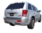
8. When you have everything in place, firmly tighten all bolts and clamps down securely. Start from the front of the vehicle and work your way to the back. Use stainless steel cleaner and a Scotch Brite pad weekly to prevent tip from discoloration. Inspect all fasteners after 25-50 miles of operation and re-tighten as necessary.
