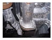
**2.** Install head pipe #A onto your existing stock front pipe and attach with bolt kit #G.
