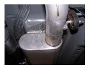
**4.** Install extension pipe #C into the muffler 1½-2". Insert welded hanger into rubber grommet. Secure to muffler with clamp #F. DO NOT TIGHTEN.
