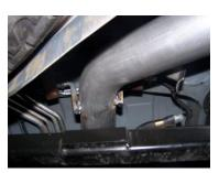
Install extension pipe #C into the muffler  $1\frac{1}{2}$ -2". Insert welded hanger into rubber grommet. Secure the muffler using clamp #F. DO NOT TIGHTEN.
