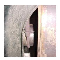
LAY OUT THE GIBSON EXHAUST ON THE FLOOR AND COMPARE PART #'S TO THE MANUAL, TO REMOVE YOUR OLD EXHAUST, CUT OFF THE TAILPIPE JUST BEHIND THE MUFFLER. NEXT REMOVE THE CLAMP LOCATED JUST IN FRONT OF THE MUFFLER THEN REMOVE YOUR STOCK MUFFLER LEAVE ALL GROMMETS IN PLACE, USE WD-40 TO AID IN REMOVAL.
