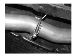
INSTALL OVERAXLE TAILPIPE #B INTO MUFFLER 1-1/2" TO 2" AND ATTACH TO MUFFLER USING HANGER #E. RE-INSTALL STOCK REAR HANGER BRACKET. USE CLAMP #G TO SECURE TAILPIPE TO HANGER. DO NOT TIGHTEN.
