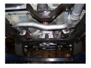
4. Install Y Pipe #A onto the stock flanges using the stock gaskets and hardware. Do not tighten. Insert welded hanger into rubber grommet.
