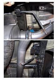
**4.** INSTALL OVERAXLE TAILPIPE # C INTO MUFFLER 1½"-2". INSERT WELDED HANGERS INTO RUBBER GROMMETS. SECURE TO THE MUFFLER USING CLAMP # E. DO NOT TIGHTEN.
