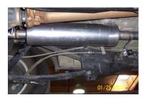
**INSTALL MUFFLER #B** ONTO HEADPIPE #A WITH **INLET TOWARDS THE** MOTOR. INLET OF MUFFLER IS LOOKING INTO THE LOUVERS USE CLAMP #E TO SECURE MUFFLER TO THE HEADPIPE, DO NOT TIGHTEN. OUTLET OF MUFFLER SHOULD BE AT THE 10 O'CLOCK POSITION.
