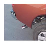
INSTALL YOUR STAINLESS TIP TO YOUR DESIRED LOOK. NOW GO BACK AND TIGHTEN ALL YOUR FLANGES, CLAMPS, ETC. STARTING FROM THE FRONT AND WORKING YOUR WAY BACK. TO CLEAN YOUR STAINLESS TIP USE A STAINLESS CLEANER AND A SCOTCH BRITE PAD. AFTER 20-25 MILES CHECK AND RETIGHTEN ALL FASTENERS IN NESERSARY.
