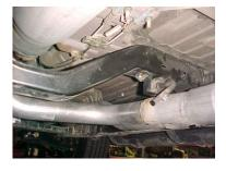
INSTALL Y-PIPE # A & I ONTO STOCK FLANGES USE YOUR STOCK HARDWARE TO SECURE. INSERT WELDED HANGER INTO RUBBER GROMMET, DO NOT TIGHTEN. USE CLAMP #J TO SECURE PIPES TOGETHER. DO NOT TIGHTEN.
