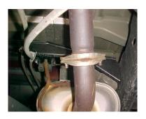
LAY OUT THE GIBSON EXHAUST ON THE FLOOR AND COMPARE PART #'S TO THE DRAWING. TO REMOVE YOUR FACTORY EXHAUST UN-BOLT YOUR TAILPIPE AT THE 2-BOLT FLANGE LOCATED BEHIND YOUR STOCK MUFFLER USE WD-40 TO AID YOU IN REMOVAL OF HANGERS FROM RUBBER GROMMETS. DO NOT DAMAGE THE GROMMETS, THEY WILL BE USED TO INSTALL THE NEW KIT
