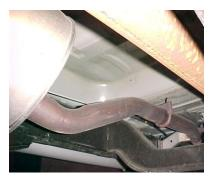
TO REMOVE YOUR STOCK EXHAUST REMOVE IT FROM THE CLAMP LOCATED JUST IN FRONT OF YOUR STOCK MUFFLER.
