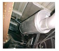
INSTALL THE MUFFLER ONTO THE HEADPIPE 1" TO 2". THE INLET OF THE MUFFLER WILL HAVE THE INSIDE LOUVERS FACING FORWARD, USE CLAMP **#D TO SECURE** MUFFLER TO THE HEADPIPE. OUTLET SHOULD BE AT THE 9 O'CLOCK POSITION. DO NOT TIGHTEN. MUFFLER INLET IS LOOKING INTO LOUVERS.
