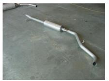
LAY OUT THE GIBSON EXHAUST ON THE FLOOR AND COMPARE PART NUMBERS WITH THE MANUAL. LEAVE ALL FACTORY GROMMETS IN PLACE. FOR EASIER REMOVAL OF GROMMETS AND HANGERS USE WD-40 ON THEM.
