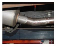
INSTALL HEADPIPE #A ONTO STOCK PIPE 1-1/2" TO 2". THE END OF THE PIPE WILL FACE UP. USE CLAMP #E TO SECURE HEADPIPE TO STOCK PIPE. DO NOT TIGHTEN.
