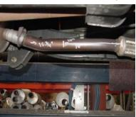
LAY OUT THE GIBSON EXHAUST ON THE FLOOR AND COMPARE PART NUMBERS WITH THE DRAWING. **TO REMOVE STOCK EXHAUST MEASURE 10 ¾" FROM THE FRONT OF THE MUFFLER TOWARDS THE MOTOR,** CUT THE TAILPIPE OFF IN THAT SPOT. REMOVE THE REAR HANGER AND SAVE THE FACTORY HARDWARE YOU WILL RE-USE IT. LEAVE ALL RUBBER GROMMETS ON THE HANGER. USE WD-40 TO AID IN REMOVAL OF THE EXHAUST AND HANGERS.
