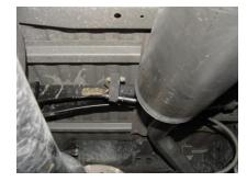
INSTALL THE MUFFLER ONTO THE HEADPIPE 1" TO 2". THE INLET OF THE MUFFLER WILL HAVE THE INSIDE LOUVERS FACING FORWARD. USE CLAMP **#D TO SECURE** MUFFLER TO THE HEADPIPE. OUTLET SHOULD BE AT THE 9 O'CLOCK POSITION. DO NOT TIGHTEN. MUFFLER INLET IS LOOKING INTO LOUVERS.
