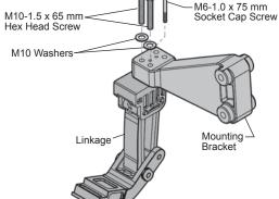
Install Linkage Assembly
