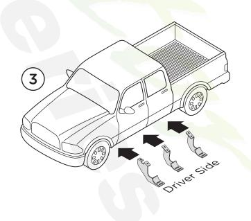
**4.** Align the Front, Center and Rear Driver's Side Brackets with the indicated holes located on the Rocker Panel of the vehicle.
