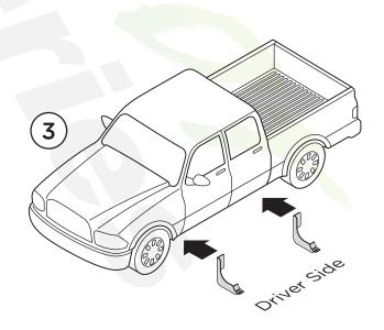
**3.** Install the Plastic Push Nut onto the Bolt Plate shown (3a). Install the Driver Side Bolt Plate into the hole in the frame (3b). The Plastic Push Nut prevents the bolt from falling into the frame and keeps the bolt straight (3c).
