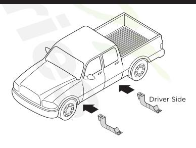
**4.** Align Front Mount Bracket with hole on underside of vehicle (4a) and fasten using one (1) Cab Mount Bolt (4b). Repeat for Rear Bracket.
