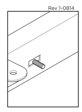
**5.** Fasten the Front Bracket to the M14 x 130MM Hex Head Bolt installed in the previous step using one (1) M14 Lock Washer, one (1) M14 Flat Washer and one (1) M14 Hex Head Nut.
